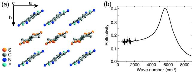
FIG. 1 (color online). (a) The crystal structure of one-dimensional organic salt ET-F<sub>2</sub>TCNQ (yellow, ET; blue, F<sub>2</sub>TCNQ). (b) Static reflectivity of the compound with electric field parallel to crystallographic *a* axis (along the ET chain).
