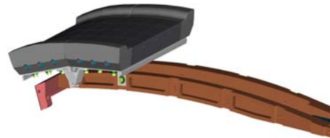
Fig. 7. TDU-SE single graphite module mounted on stainless steel support truss
