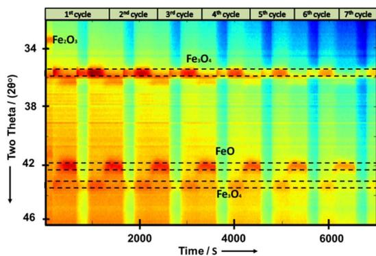
Figure 6. Time resolved 2D in-situ XRD pattern during 7 redox cycles at 650 °C for FeAl90:10.
