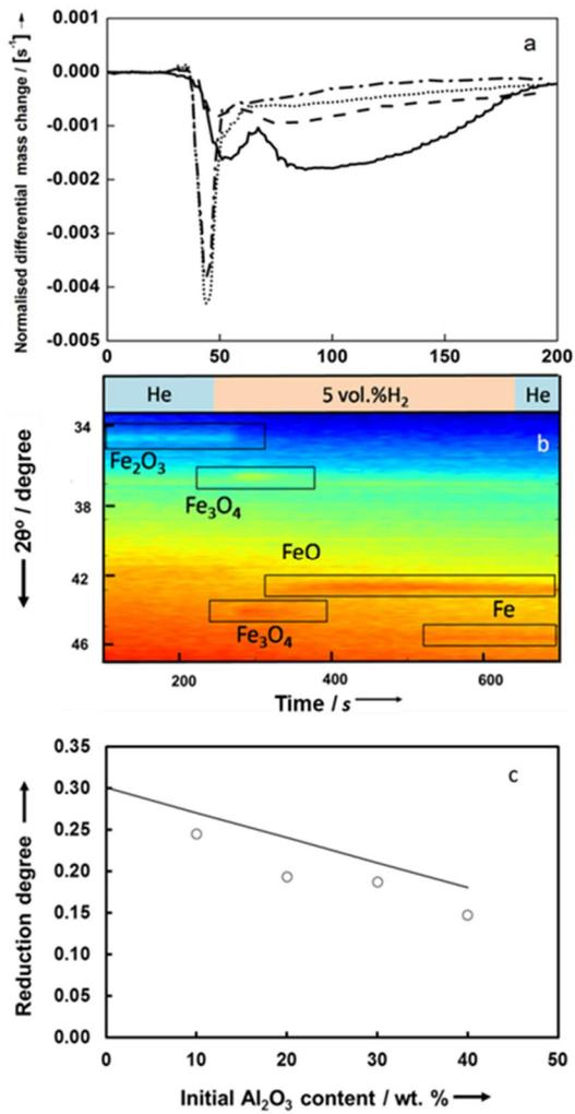
**Figure 2.** (a) differential mass loss during isothermal reduction by H<sub>2</sub> at 800 °C. solid: FeAl90:10, dashes FeAl80:20, dots: FeAl70:30, dash-dots: FeAl60:40, (b) Time resolved XRD pattern during reduction at 750 °C of FeAl90:10, (c) theoretical (straight line) and observed reduction degree (○) from TGA for all FeAl samples.
