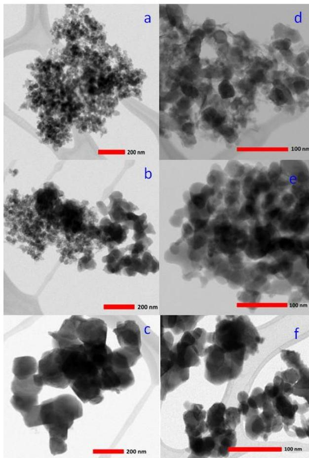
**Figure 10.** STEM images of (a) fresh FeAl90:10, and post reaction images after (b) 7 and (c) 100 cycles; The STEM images of FeAl70:30:(c) fresh and after exposure to alternating H<sub>2</sub> and CO<sub>2</sub> environment after (e) 7 and (f) 100 cycles.
