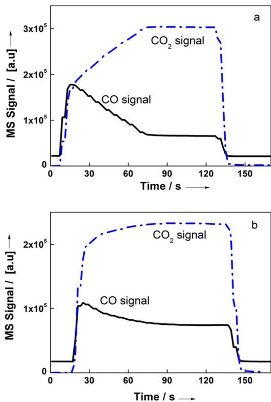
Figure 3. MS signals for CO<sub>2</sub> and CO, (a) first of 100 chemical looping cycles with alternating H<sub>2</sub> and CO<sub>2</sub> feed (b) 100<sup>th</sup> cycle for the sample Fe90:10 at 750 °C.
