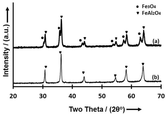
**Figure 9.** XRD pattern for the sample FeAl70:30 after 100 redox cycles (a) at 650 °C and (b) at 750 °C.
