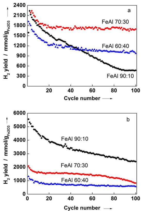
Figure 5. H<sub>2</sub> yield over 100 cycles for FeAl90:10, FeAl70:30 and FeAl60:40; at reaction temperature (a) 650 °C and (b) 750 °C.
