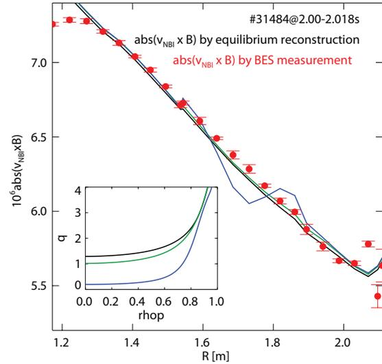
Figure 4: Measured  $\mathbf{v}_{NBI} \times \mathbf{B}$  profile compared with equilibrium reconstructions.
