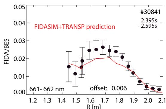
Figure 7: *Radial FIDA profile, normalized by the beam emission intensity and compared with the prediction from FIDASIM+TRANSP*
