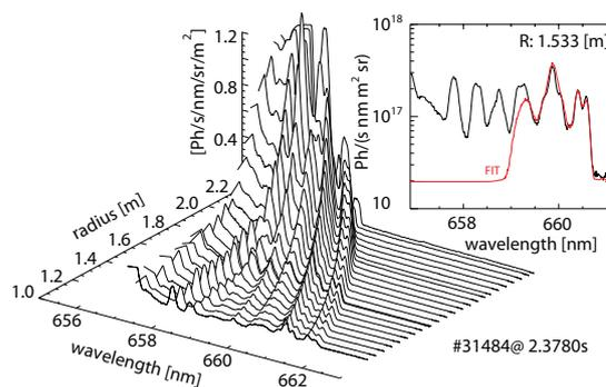
Figure 3: Measured beam emission as a function of radius and wavelength.
