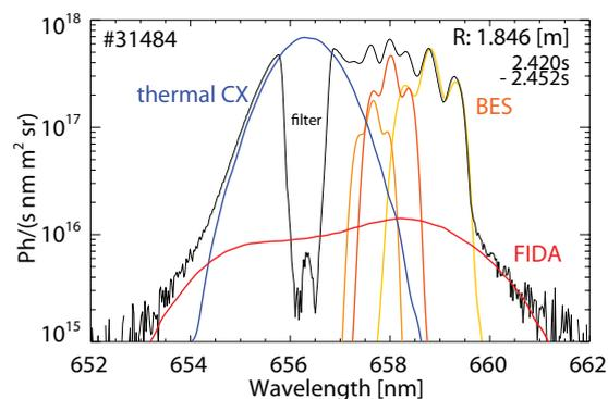
Figure 1: Measured and simulated active Balmer alpha spectrum.
