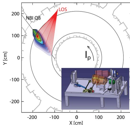
Figure 2: Top-down view showing the LOS setup in red and a contour plot of the neutral density during operation of NBI Q8.
