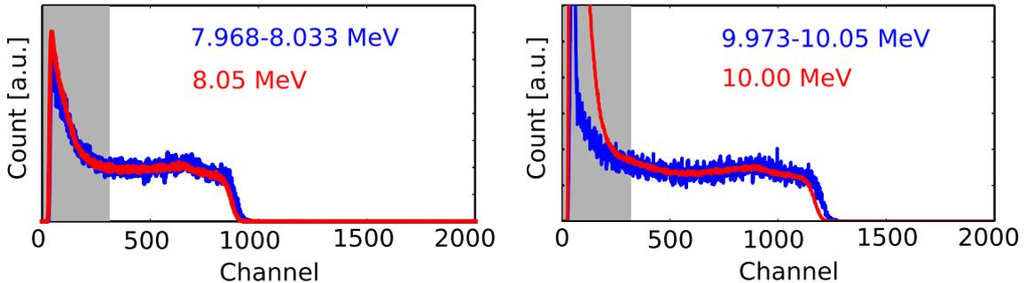
Figure 2 . Detector response at  $E_n=8$  and 10 MeV. Selecting energy interval from time-of-flight measurement (blue), monoenergetic (red).
