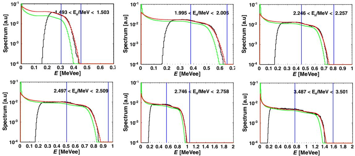
Figure 1 . Detector response at several energies. Measured (black), simulated (green), optimised (red). The blue vertical lines delimit the region used for the fit.
