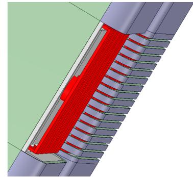
**FIGURE 2.** Antenna (Faraday Screen partially removed)
