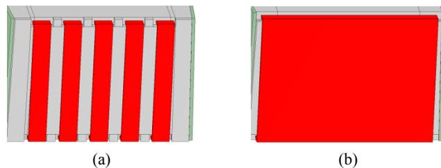
**FIGURE 3.** Covering ratio of the antenna straps: 49% (a) and 94% (b)
