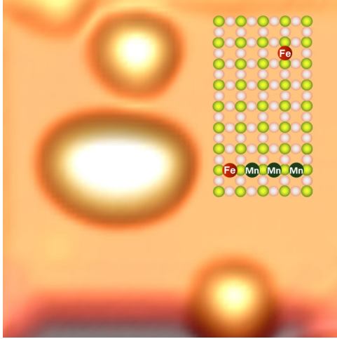
FIG. 1. Constant current STM image of a \text{FeMn}_3 chain assembled on a \text{Cu}_2\text{N} layer and atomic scheme (on the right of the figure) that can be inferred from the position of the upper-right Fe atom and manipulation with the STM tip. The STM image was scanned at 10 mV and 100 pA. The scanned area is 6 \times 6 \text{ nm}^2 . The transition-metal atoms were always placed on top of a Cu atom between two nitrogen atoms. The topography was processed with WSXM [25].
