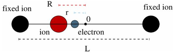
FIG. 1. Schematic representation of the model proton-coupled electron transfer.
