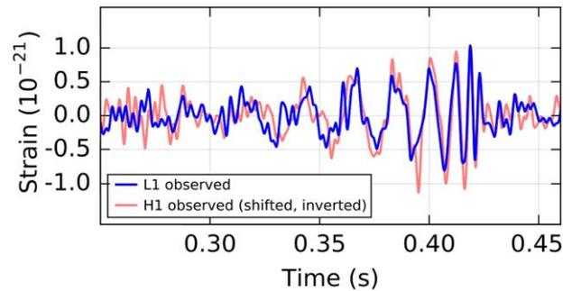
**Figure 1** The instrumental strain data in the Livingston detector (blue) and Hanford detector (red), as shown in Figure 1 of [1]. Both have been bandpass- and notch-filtered. The Hanford strain has been shifted back in time by 6.9 ms and inverted. Times shown are relative to 09:50:45 Coordinated Universal Time (UTC) on September 14, 2015.
