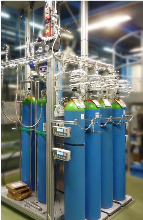
(a) Filling and recuperation side. On the right there are the 4 filling bottles and on the left the 2 recuperation bottles.
