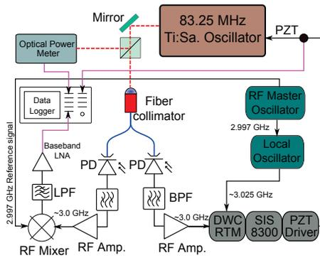
Figure 2: Detailed block diagram of DWC based locking setup with out-of-loop phase detector.
