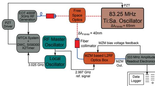
Figure 4: The block diagram of the MZM based laser to RF phase detector measurement setup.
