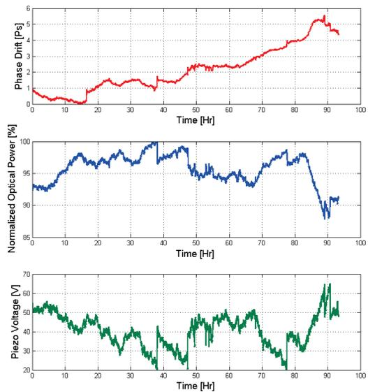
Figure 3: Measurement of long term out-of-loop phase stability, optical power and piezo voltage.
