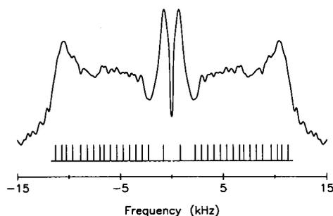
FIGURE 1 Depaked 46.1 MHz  $^2H$  NMR spectrum of 1-stearoyl-2- $[^2H_{33}]$ stearoyl-*sn*-glycero-3-phosphoethanolamine dispersed in 2.4 M NaCl and recorded at 97°C. The dePaked display corresponds to resonances for the magnetic field oriented parallel to the ordering axis. The stick plot represents contiguous sections of the spectrum whose intensities correspond to a single  $CD_2$  groups, and is defined according to the convention of Sternin et al. (1988).
