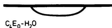
FIG. 2. Profile of a lens of n -butanol ( C_4E_0 ) floating at the interface between water saturated with butanol and air at 25 °C, copied from a photograph.
