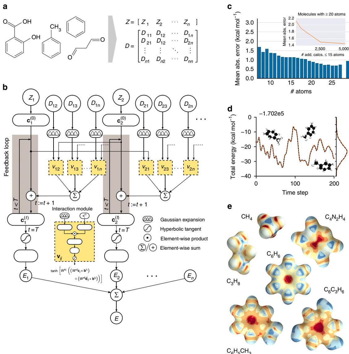
**Figure 1 | Prediction and explanation of molecular energies with a deep tensor neural network.** (a) Molecules are encoded as input for the neural network by a vector of nuclear charges and an inter-atomic distance matrix. This description is complete and invariant to rotation and translation.
