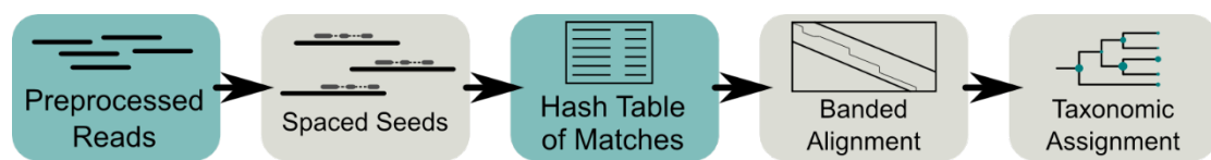
Figure 1 – Schematic overview of MALT. For each preprocessed metagenomic sequencing read, the algorithm generates all contained spaced seeds and looks them up in a hash table of spaced seeds representing the reference database. A banded alignment is calculated for each match of seeds. Once all alignments for a given read have been calculated taxonomic binning of the read is performed using the LCA algorithm.
