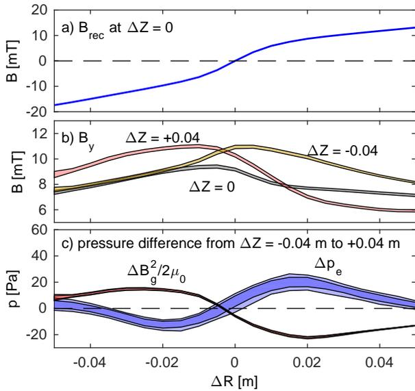
FIG. 3. Radial profiles of (a) the reconnecting component of magnetic field at  $\Delta Z = 0$ ; (b) out-of-plane field  $B_y$  at  $\Delta Z = -0.04$  (red), 0 (gray), and  $+0.04$  m (yellow); (c) electron pressure (blue) and guide field pressure (red) differences between  $\Delta Z = -0.04$  and  $+0.04$  m. Measurements are at positive GF ( $B_g = +0.8B_{up}$ ).
