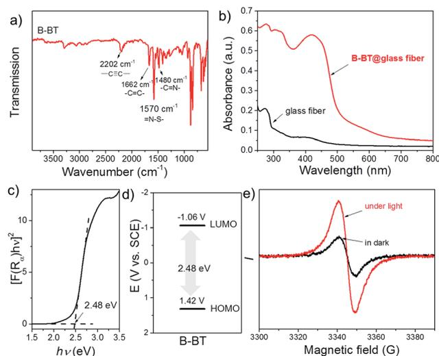
**Fig. 2** (a) FT-IR spectrum of B-BT, (b) diffuse reflectance (DR) UV/Vis spectra of pure and B-BT-coated glass fibers, (c) Kubelka–Munk-transformed reflectance spectrum of B-BT, (d) HOMO and LUMO positions of B-BT, and (e) EPR spectra of B-BT in the dark and under visible light irradiation.
