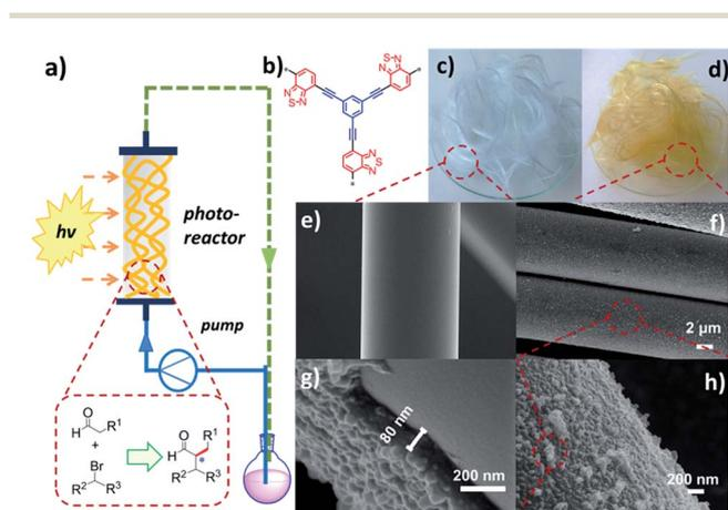
**Fig. 1** (a) An illustrated setup of a fixed-bed photoreactor using conjugated nanoporous polymer-coated glass fibers. (b) Molecular structure of B-BT. (c) Photography of pure glass fibers and (d) B-BT-coated glass fibers. (e) SEM images of pure glass fibers and (f–h) B-BT-coated glass fibers.
