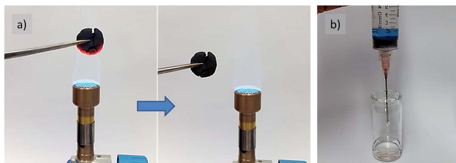
Fig. 6 Images of the nitrogen-doped carbon cookie made from glucose–urea–salt with 39 wt% of cellulose carbonized at 500 °C (a) monolith during repeated firing cycles using a butane/propane gas burner and (b) powder during sorption of methylene blue dye from aqueous solution.
