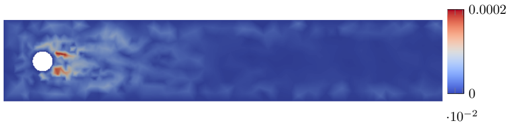
Fig. 10 Absolute error in |v| obtained from the full-order and reduced-order systems on the full grid.
