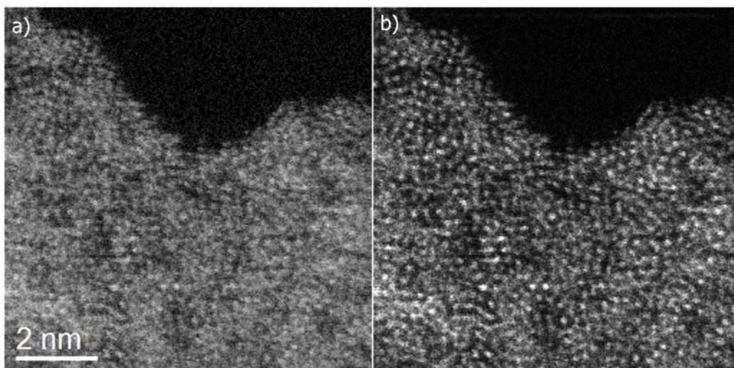
Figure S2. a) Original HAADF and Fourier filtered HAADF images of the IrO<sub>x</sub>-FHI.
