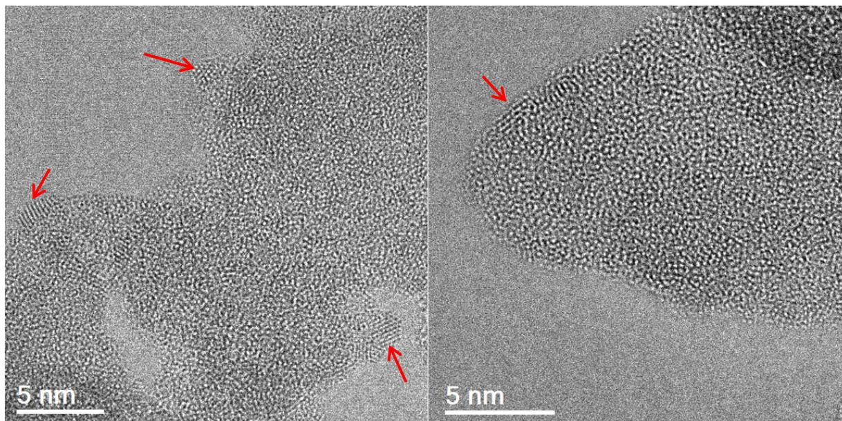
Figure S9. HRTEM images of  $\text{IrO}_x$  hydroxides showing formation of the Ir metallic phase (marked with red arrows) on the particle surfaces induced by e-beam irradiation.
