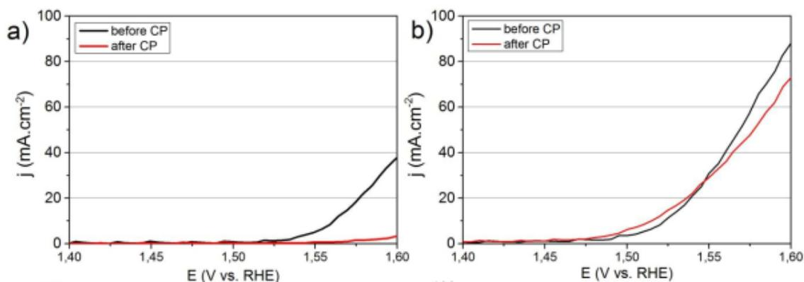
Figure S1. Linear sweep voltammetry measurements (5 mV.s<sup>-1</sup>) before (black line) and after the 2h-stability test (red line): a) IrO<sub>x</sub>-commercial; b) IrO<sub>x</sub>-FHI.<sup>1</sup> The stability test was performed using chronopotentiometry (CP) measurements at 10 mA/cm<sup>2</sup> for 2 hours.
