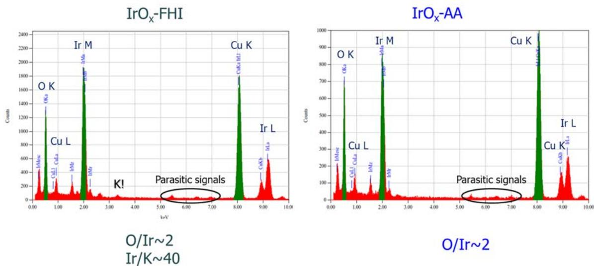
Figure S4. EDS analysis of elemental composition Ir hydroxides.
