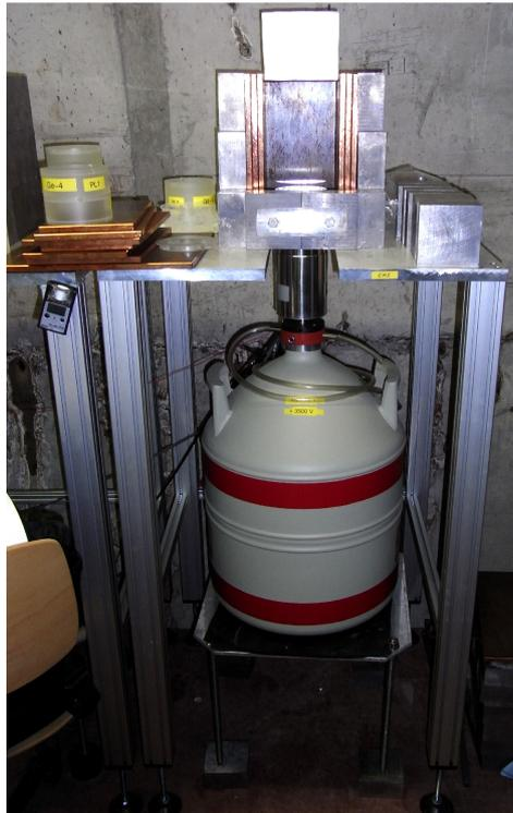
**Figure 2.5:** The Heidelberg table for fixed calibration source measurements with positioned detector in vacuum cryostat. The lead and copper shieldings are opened, the plastic source holders are shown left to the shielding.
