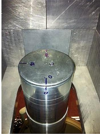
**Figure 3.2:** Picture of a detector's cryostat with the modified Pb plate used for the collimated <sup>241</sup>Am top scans to investigate the  $A/E$  position-dependence.
