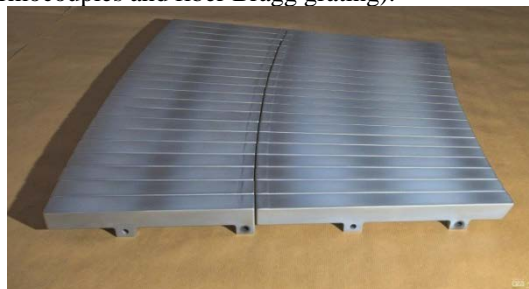
Figure 2: Start up graphite tiles for WEST lower divertor after W coating
