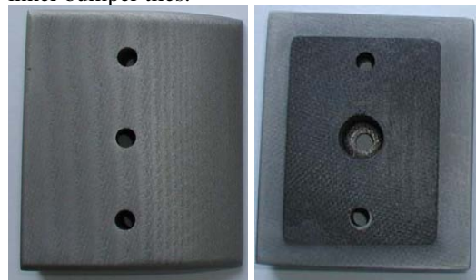
Figure 7: Inner bumper CFC tile with W coating: front and bottom face
