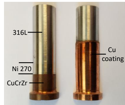
Fig. 3: un-coated and coated connectors
