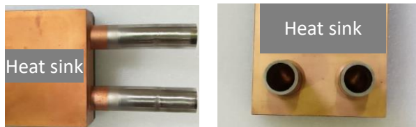
Fig. 1: position of water connectors of target element
