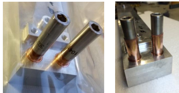
Fig. 4: test connectors mounted on dummy Al target element before (left) and after coating (right)
