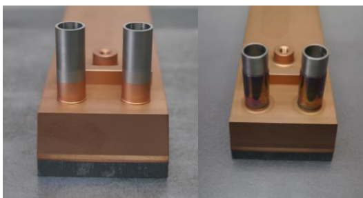
Fig. 7: connectors of series target element before and after coating
