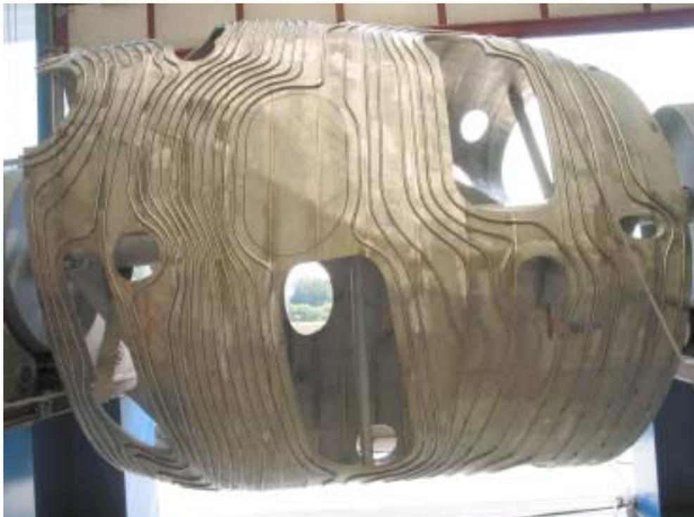
Figure 2: 27° half module sector with assembled heating and cooling pipes
