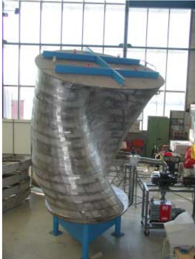
Figure 1: Integral helium-leak-test of a 27° half module sector
