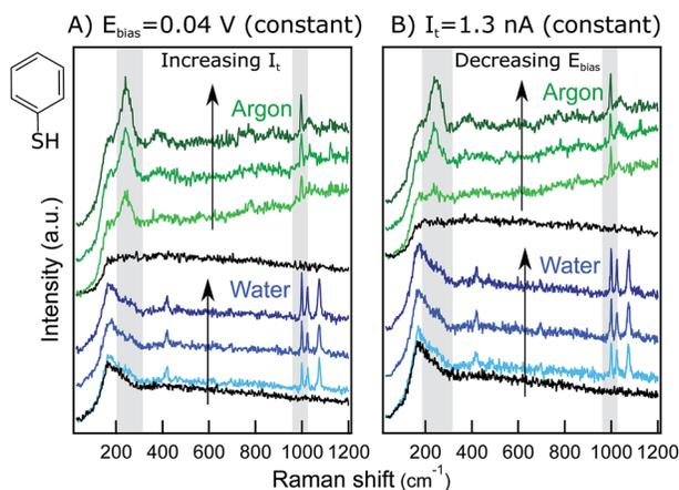
Fig. 1 Raw spectra recorded in Ar (green) and in water (blue) for (A)  $I_t$  ramped at a constant  $E_b$  of 0.04 V, (B)  $E_b$  ramped at a constant  $I_t$  of 1.3 nA. For each series, 20 nm retraction spectra (far-field) are included in black. Gray rectangles indicate marker bands. Spectra are y-offset for clarity. Inset: PhS chemical structure.
