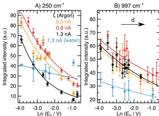
Fig. 3 (A) Integrated intensity of the 245  $\text{cm}^{-1}$  mode ((B) 997  $\text{cm}^{-1}$ ) as a function of  $E_b$  at constant  $I_t$  values of 0.3 nA (orange triangles), 0.8 nA (red circles), and 1.3 nA (black squares) in Ar and 1.3 nA in water (light blue diamonds). Averaged results from spectra taken in scans up and down are presented with the standard deviations as the errors. Fittings to eqn (3) are included (solid lines).
