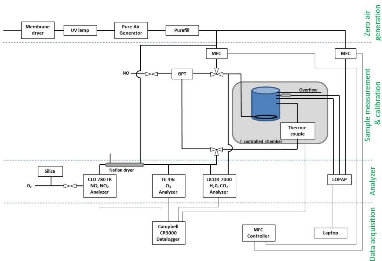
**Figure S3:** Schematic overview of the setup used to measure  $F(\text{HONO})$  and  $F(\text{NO})$ . It can be separated into zero air generation, measurement and calibration, analyzer, and data acquisition.
