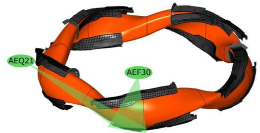
Figure 1: Sketch of the two views of the CIS diagnostic on W7-X.
