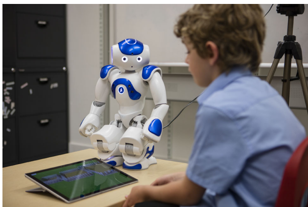
Fig. 2 The L2TOR setup includes the NAO robot standing to the side of the child with a tablet in between them
