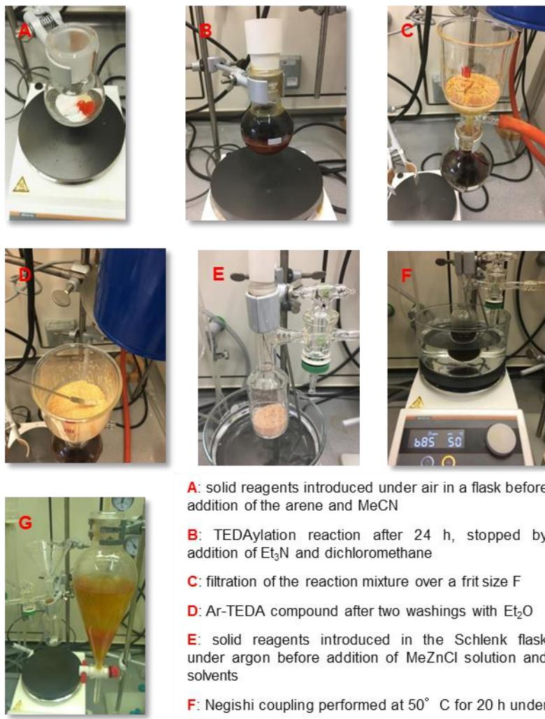
**A:** solid reagents introduced under air in a flask before addition of the arene and MeCN
