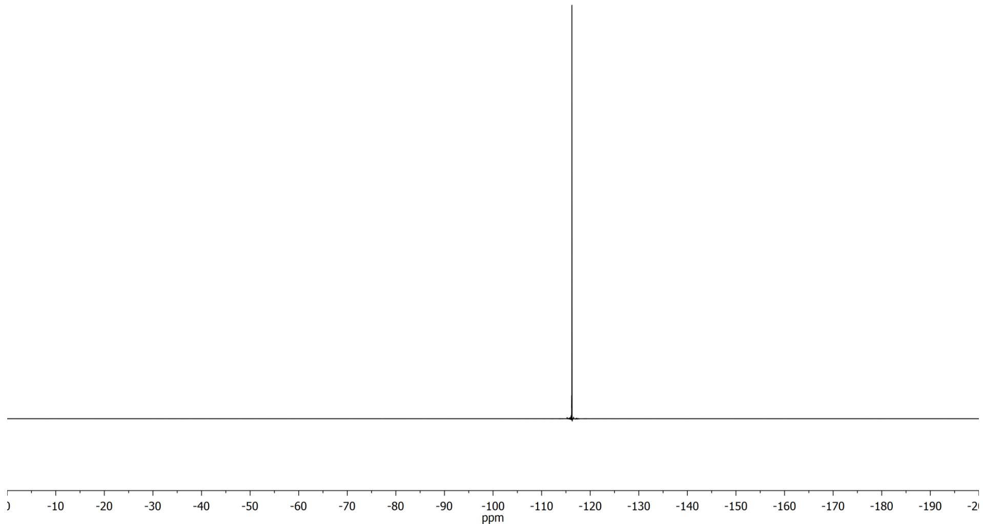
**<sup>13</sup>C NMR of 4-fluoro-4'-methyl-1,1'-biphenyl (4e)**CDCl<sub>3</sub>, 23 °C
