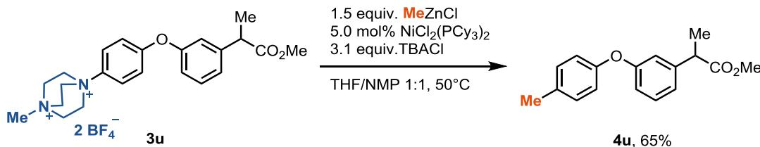
In an anhydrous, nitrogen-filled glovebox, a 4 mL vial was charged with Ni(PCy<sub>3</sub>)<sub>2</sub>Cl<sub>2</sub> (8.6 mg, 12 µmol, 5.0 mol%), **3u** (139 mg, 0.250 mmol, 1.00 equiv.), and *n*Bu<sub>4</sub>N<sup>+</sup>Cl<sup>-</sup> (215.4 mg, 0.77 mmol, 3.10 equiv). NMP (0.75
