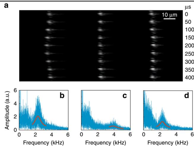
**Fig. 3** Thermally driven collective motion of the bound-particle array. **a** A series of snapshots of the bound-particle array during one period of the breathing mode, captured with a high-speed camera. **b–d** Spectra for the mechanical motion of the three bound particles. The blue curves are the measured data, and the red curves are the Lorentzian fits
