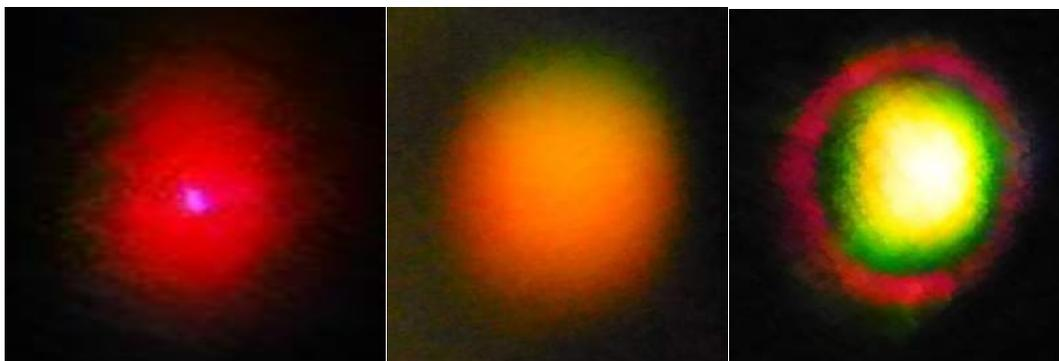
Figure 2.7: Stages of SC development, "first light" Third Harmonic (left), Third Harmonic and AS peak (center), fully broadened SC (right), from the ICFO  $1.8\mu\text{m}$ -pumped experiments in YAG.
