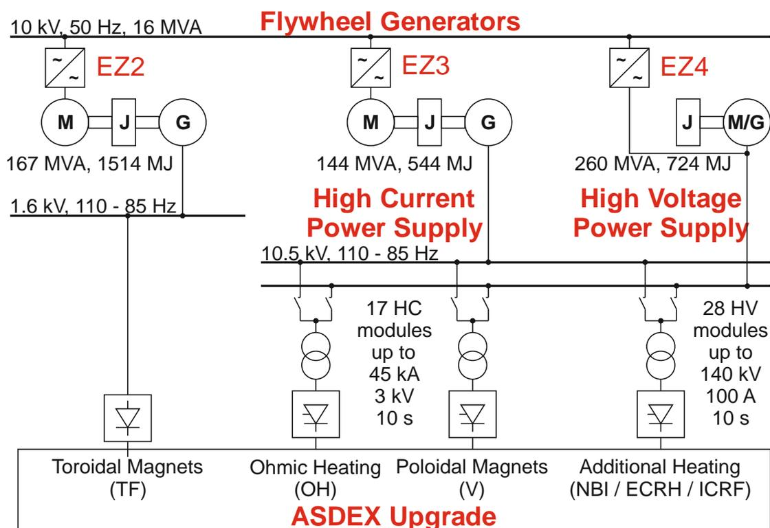
Fig.1: Fusion experiment power supply network
