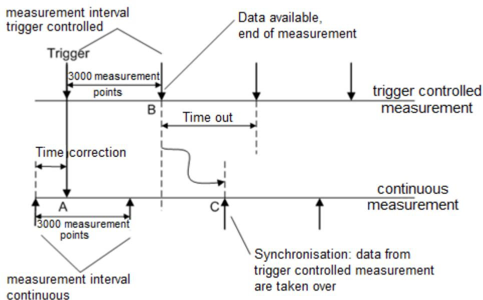
*Fig.5: Synchronization of trigger based and continuous measurements*
