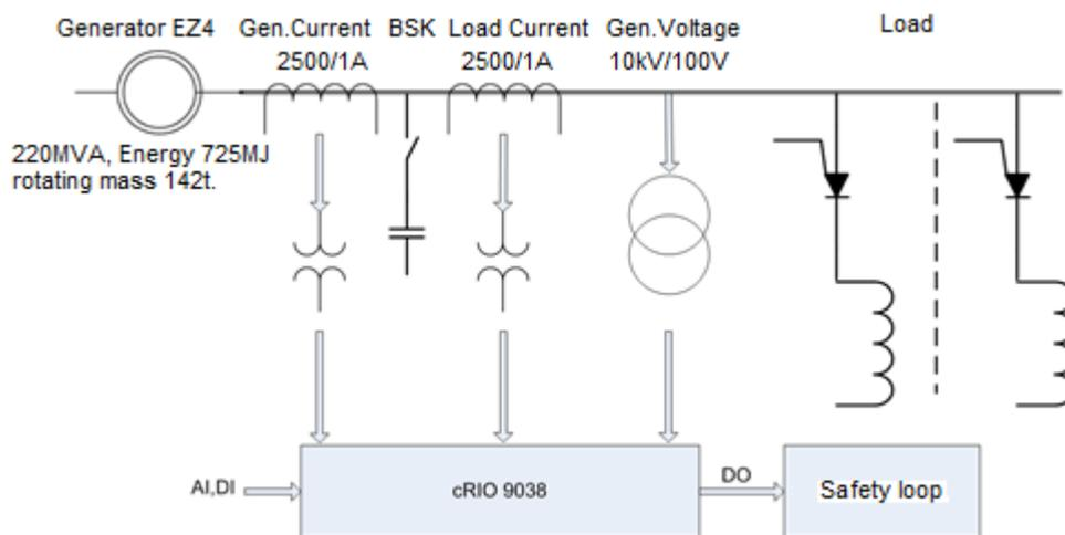
Fig. 4: Supervising system of generator EZ4 with input and output signals
