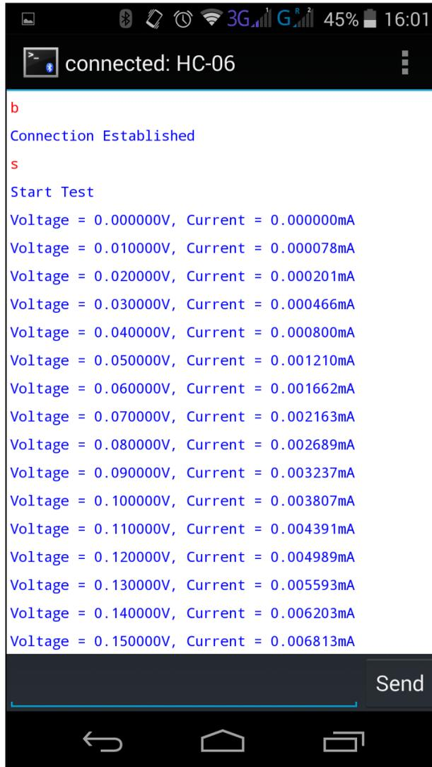
**Figure S5.** A screenshot of Bluetooth terminal shows data received by the Smartphone during a test demonstrating communication between device and phone.
