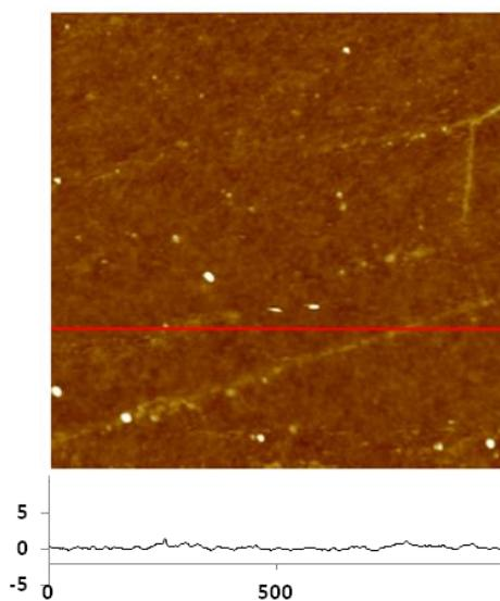
**Figure S2.** AFM images of graphene transistor surface without the DNA sensor in air. The graphene surface is mostly flat with some wrinkles. Surface height profiles at the red line are plotted at the bottom of each image. Unit is nm.
