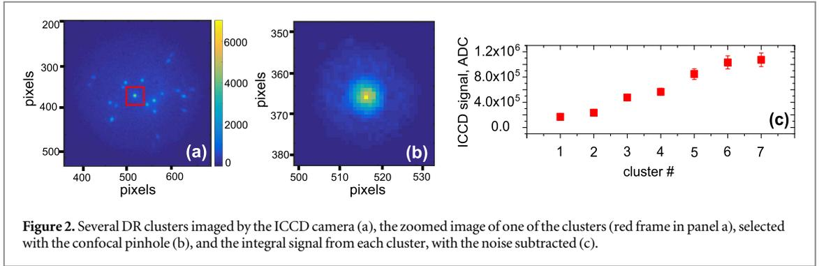
**Figure 2.** Several DR clusters imaged by the ICCD camera (a), the zoomed image of one of the clusters (red frame in panel a), selected with the confocal pinhole (b), and the integral signal from each cluster, with the noise subtracted (c).
