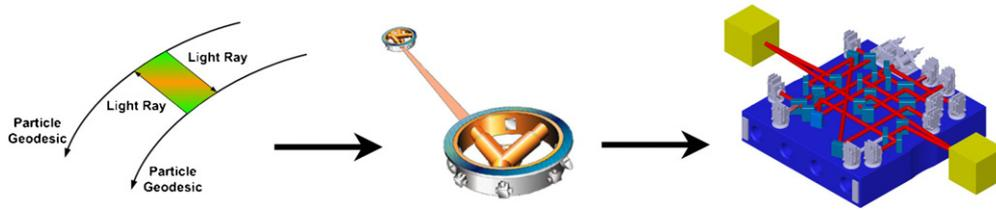
**Figure 1.** The classical Einstein gedankenexperiment (left), one arm of LISA showing the relationship to the gedankenexperiment (middle) and LISA technology package, showing the two free-floating test masses and the laser interferometer (right).
