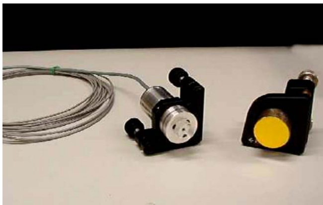
FIGURE 3 Comparison between piezo actuated mirrors (left) and static test mirrors (right)
