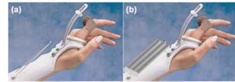
Fig. 1. Dynamic hand splints: (a) a state-of-the-art example of passive splint equipped with an elastic band; (b) schematisation of the concept here proposed, consisting in the substitution of the passive elastic band with active elastic actuators.
