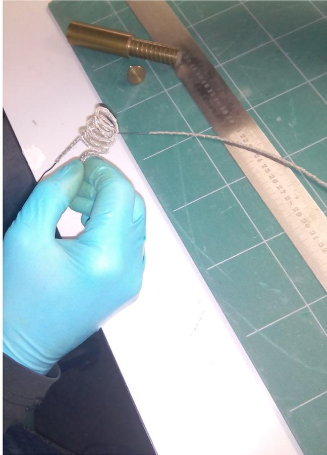
Figure 5: Coiled ion source filament before coating. In the background, the grooved brass cylinder used to coil the filament and an uncoiled tantalum filament, already wrapped in a nickel mesh, can be seen.
