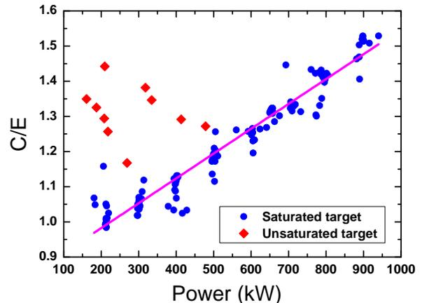
FIG. 5: Ratio  $C/E$  between the calculated and measured neutron emission as a function of the power on the dump
