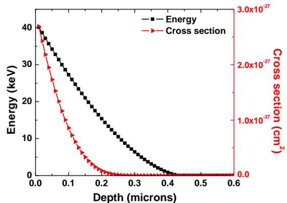
FIG. 2: Deuteron energy (left scale) and the  $D(d, n)^3He$  cross section (right scale) as a function of depth at 40 keV
