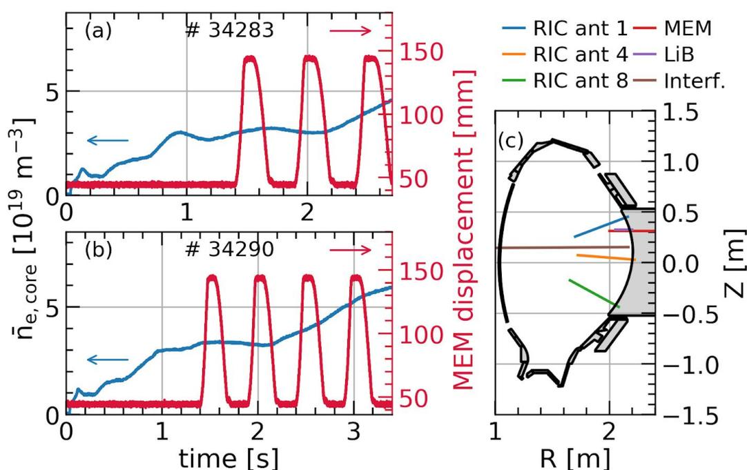
Figure 1. Left, Temporal evolution of line averaged core electron density (blue) and MEM displacement (red) for discharges (a) #34283 ( $I_p = 600 \text{ kA}$ ) and (b) #34290 ( $I_p = 800 \text{ kA}$ ). Right (c), poloidal cross-section of AUG together with line of sights of: RIC antenna 1/4/8 (blue/orange/green), MEM (red), LiB (purple), core interferometry (brown).
