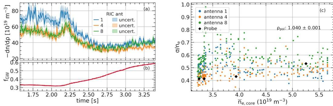
Figure 3. Left, on the top evolution of profile gradients (and statistical uncertainty) in discharge #34290, calculated between densities  $0.75 - 1.25 \cdot 10^{19} \text{ m}^{-3}$ , corresponding to the near SOL region; on the bottom, evolution of Greenwald fraction. Right, the fluctuation level estimated at  $\rho_{pol} = 1.04$  from RIC and MEM profiles in dependence on line averaged core electron density.
