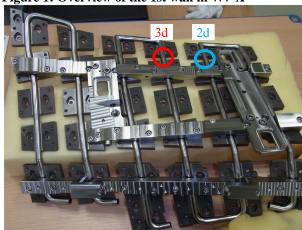
Figure 2: Baffle module 7v without graphite tiles and crack location 2d and 3d, seen from the vessel side
