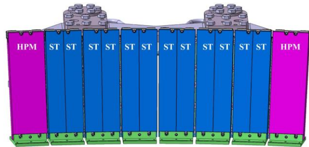
Fig. 6. CAD model the standard module installed in AUG. The outermost pink tiles are made of HPM and the remaining are the split tungsten tiles.
