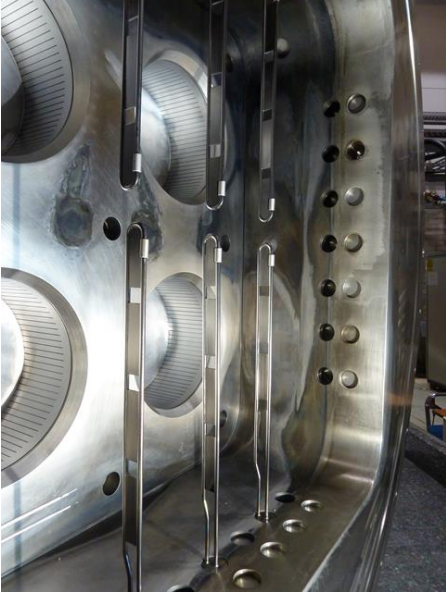
FIGURE 3. Internal potential rods used in ELISE. The rectangular openings in the rods are positioned at the location of the horizontal OES lines of sight.
