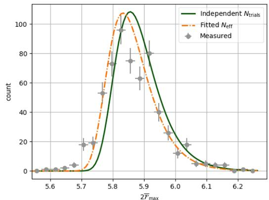
FIG. 2. The distribution of recovered  $2\bar{\mathcal{F}}_{\max}$  values in 600 repeated runs over Gaussian noise for GCT (top) and Weave (bottom). If the search templates were independent the measured  $2\bar{\mathcal{F}}_{\max}$  (grey) would agree with expected  $2\bar{\mathcal{F}}_{\max}$  for  $N_{templates}$  (green). The effective number of templates is obtained with a fit to the measured  $2\bar{\mathcal{F}}_{\max}$ , the results of the fit are shown in orange.
