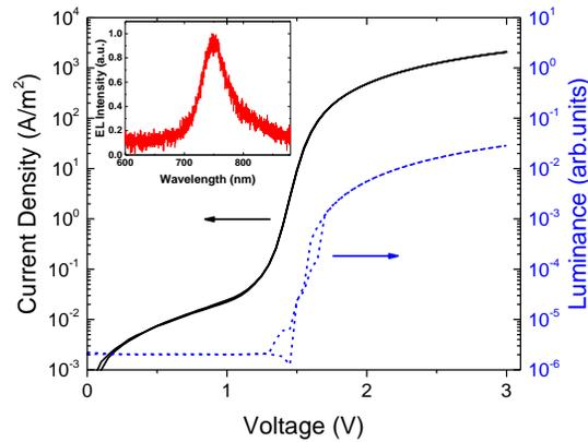
FIG. 3. Current density and luminance vs voltage for an ICBA light-emitting diode with an ICBA layer thickness of 118 nm. The electroluminescence (EL) spectrum is shown in the inset.
