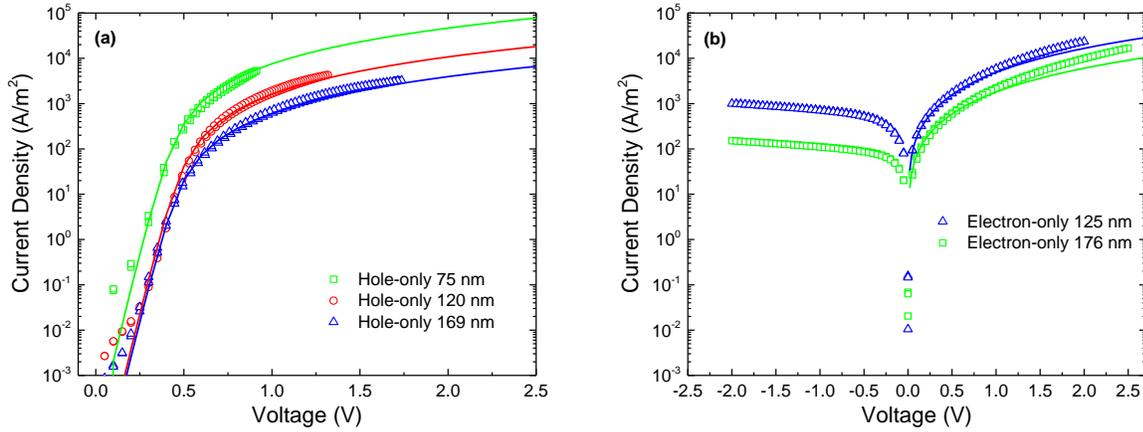
Fig. 6. Current density-voltage characteristics of ICBA hole-only (a) and electron-only (b) devices of different layer thickness. The symbols represent experimental data, the lines are fits with drift-diffusion simulations using a constant mobility.
