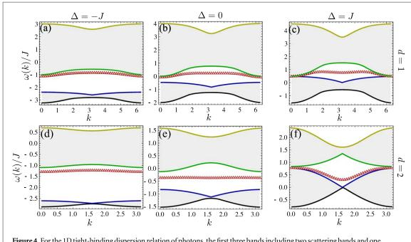
**Figure 4.** For the 1D tight-binding dispersion relation of photons, the first three bands including two scattering bands and one doublon band in the middle. (a)–(c) for d=1:  $\Delta/J=-1$ ,  $\Omega/J=1$  (a);  $\Delta/J=0$ ,  $\Omega/J=1$  (b);  $\Delta/J=1$ ,  $\Omega/J=1$  (c); (d)–(f) for d=2:  $\Delta/J=-1$ ,  $\Omega/J=1$  (d);  $\Delta/J=0$ ,  $\Omega/J=1$  (e);  $\Delta/J=1$ ,  $\Omega/J=1$  (f).
