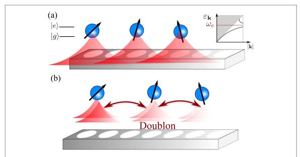
Figure 1. (a) Scheme of the model: several QEs are coupled to a structured bosonic bath with energy dispersion  $\varepsilon_{\mathbf{k}}$ . Though, we schematically plotted a 1D bath, the results can be extended to higher dimensions. (b) Pictorial representation of the doublon states hopping between QEs.
