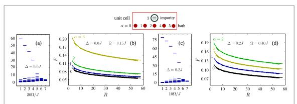
**Figure 14.** The correlation function matrix  $F_{i\alpha,j\beta}$  in the system with  $N_{\text{imp}} = N_{\text{exc}} = 80$ . The structure of a unit cell is shown on the top. Panels (a) and (c) show the 10 largest eigenvalues of  $F_{i\alpha,j\beta}$ . Panels (c) and (d) show the scaling of  $F_{i\alpha,j\alpha}$  versus R = |i-j|, where the markers are numerical values and the lines are least square fitting results.
