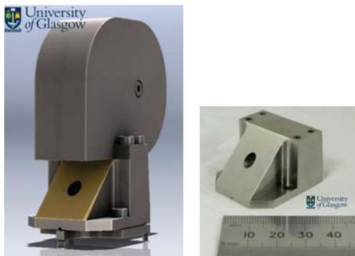
Fig. 12. Design (left) and actual reflector (right) of the TX Beam Clip. The reflection is steered to an overhead beam dump with an internal spiral minimizing any back scattering.
