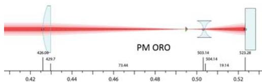
Fig. 16. Example of an alternative imaging design for the PM ORO, based on only 2 commercially available lenses.
