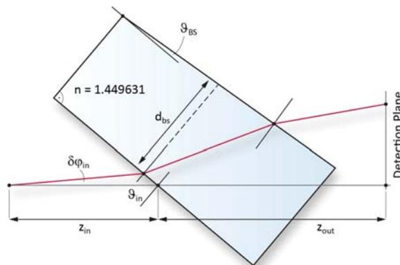
Fig. 6. Schematic illustration of the beam path through a wedged component, in the presence of pointing jitter  $\delta\varphi_{in}$ .
