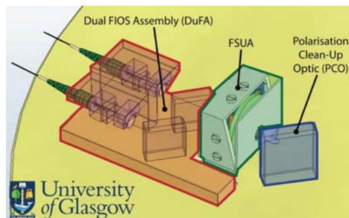
Fig. 7. Fiber Switching Unit, consisting of a Dual FIOS Assembly (DuFA), a Fiber Switching Unit Actuator (FSUA), and a polarizing beamsplitter (PCO).
