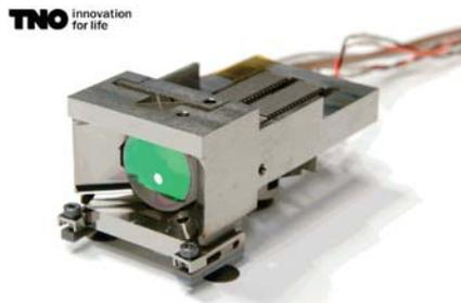
Fig. 13. Breadboard of the Point-Ahead Angle Mechanism. This design variant allows beam steering in the beam plane on the Optical Bench, i. e. the axis of rotation is perpendicular to the OB surface.
