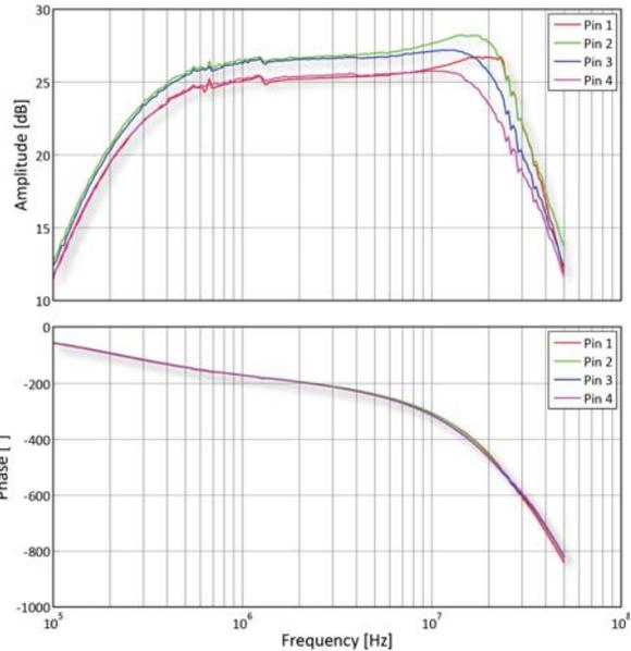
Fig. 21. Measured amplitude and phase response of the prototype transimpedance amplifier front-end.
