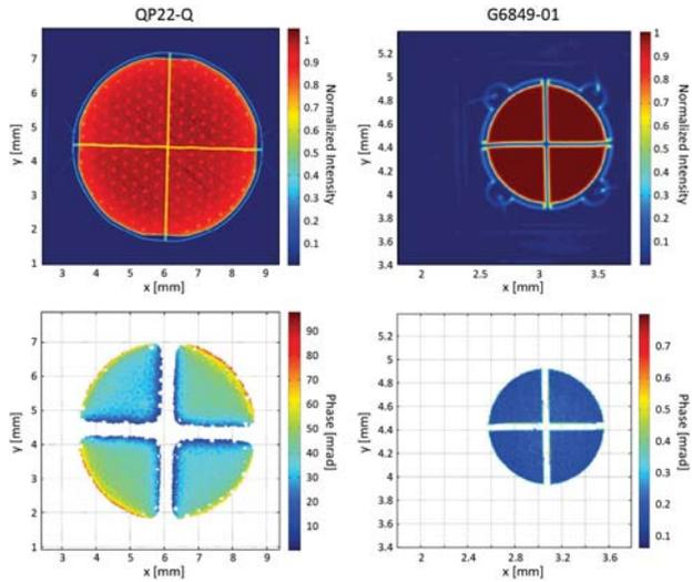
Fig. 23. Spatially resolved response for the QP22-Q and the G6849-01. The measurement was performed by scanning a pencil beam with a spot size of  $w_0 = 21 \mu\text{m}$  over the active area. For observation of the phase response, two laser frequencies separated by 10 kHz were generated within the same pencil beam, and their relative phase was referenced to a second, stable photodiode.
