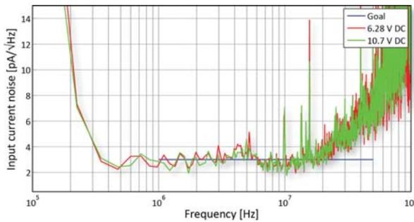
Fig. 20. Measured input current noise of the prototype trans-impedance amplifier at two different reverse voltages. The blue line indicates the design goal of  $3 \text{ pA}/\sqrt{\text{Hz}}$
