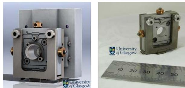
Fig. 18. Photodiode assembly consisting of a precision flexure mount for the Quadrant Photodiode and an RF enclosure for the front-end electronic. An actual prototype of the QPD mount is seen on the right.
