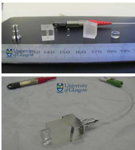
Fig. 9. The Fiber Injector Optical Subassembly is assembled from various glass elements which are joint using Hydrxoid Catalysis Bonding on all surfaces in the optical path. Various prototypes demonstrate that this can provide beams of excellent wavefront quality of  $\lambda/30$  rms or lower.
