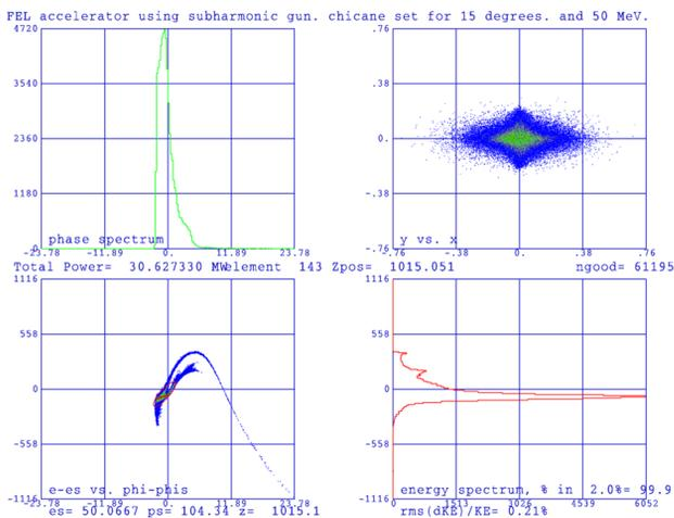
Figure 3: 50 MeV end-to-end TStep simulation at the exit of the Far-IR achromat.
