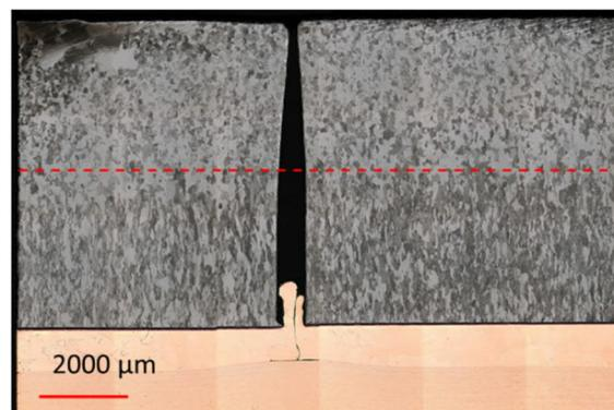
Fig 4. ENEA#11 axial cross-section after 500 cycles 20 MW/m<sup>2</sup>. The dashed red line marks the beginning of recrystallization. The total thickness of the W block is 7 mm.
