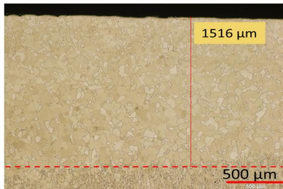
Fig 6. ENEA DEMO#5, cross-section of the centre of W block 12 after 500 cycles 20 MW/m<sup>2</sup>. The dashed red line marks the beginning of recrystallization.
