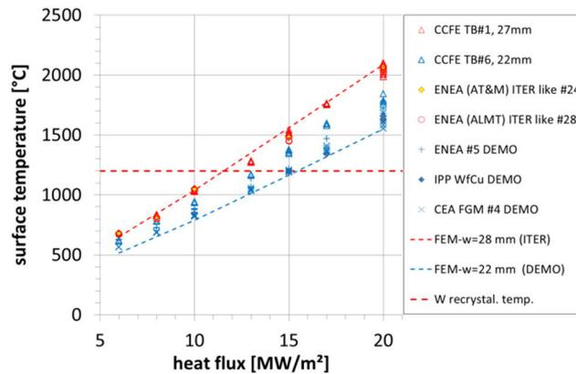
Fig. 2. Surface temperature of selected concepts depending on the incident heat flux at 130°C, 4 MPa, 16 m/s cooling water velocity. The presented temperatures were pyrometrically measured in the centre of mock-ups.
