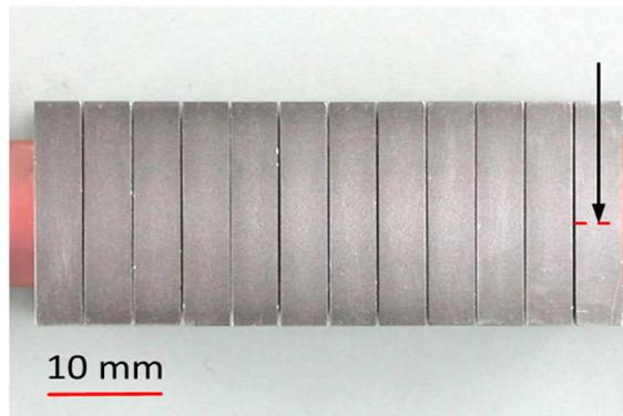
Fig 5. Surface view on ENEA DEMO #5 after 500 cycles 20 MW/m<sup>2</sup> loading at hot water cooling. The arrow marks the micrograph shown in Fig.6. The total thickness of the W block is 5 mm.
