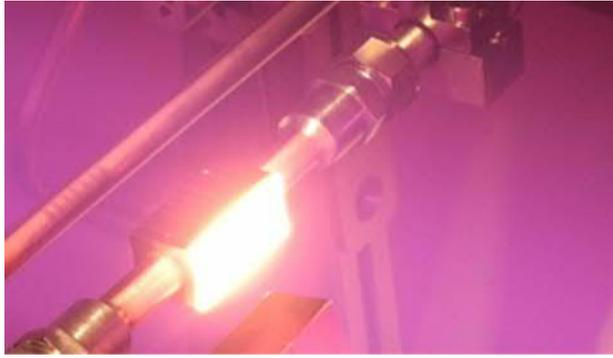
Fig. 1: Arrangement of the mock-ups in GLADIS. The image shows a DEMO type mockup made by CEA and equipped with 10 W blocks. The mock-up is fully loaded in the neutral beam at 20 MW/m<sup>2</sup>. The water connectors are protected by beam scrapers. The scraper of the water outlet (lower left in the image) is visible.
