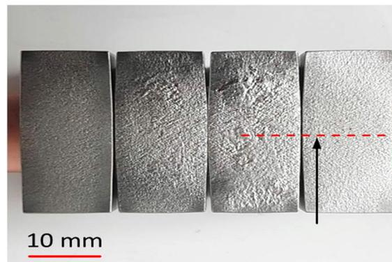
Fig. 3. Surface view on ENEA ITER like #11 after 500 cycles 20 MW/m<sup>2</sup> loading at hot water cooling. The position of the micrograph shown in Fig. 4 is marked by the dashed line.
