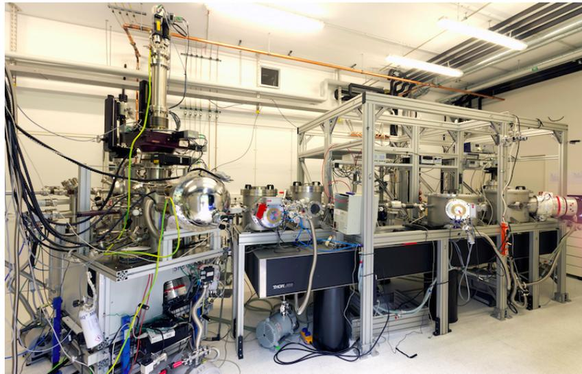
**Figure 2.3:** XUV beamline at Hamburg consisting of 4 vacuum chambers holding a gasjet, a grating, a slit and 3 toroidal mirrors.
